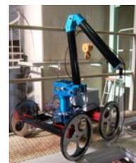
Fig.1. Measurement system with conveying robot and phased array sensor.
