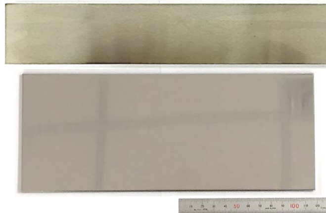
Fig. 2. RAFM-ODS steel sheet with a thickness of 1 mm.
