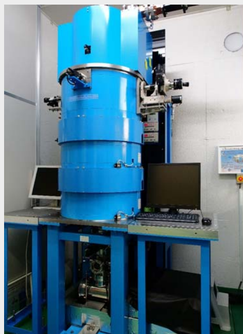
Figure 1: The prototype of relativistic-energy UEM using a photocathode RF gun
