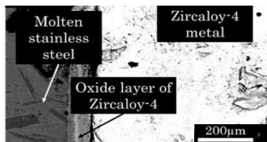
Fig.1 Cross sections of sample heated at 1300°C for 60 min in H 2 O/Ar atmosphere using Zircaloy-4
