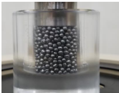
Fig. 1 Single-sized Be 12 V pebbles in a cylindrical container
