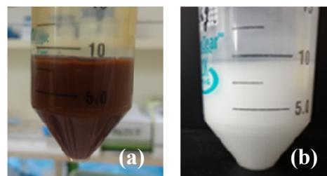
Fig.1 Simulated iron co-precipitation slurry (a) and carbonate salt slurry (b) [4]
