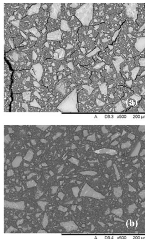
Fig.2 BSE images of phosphate cements: (a) cured at 35°C and (b) 95°C [5]
