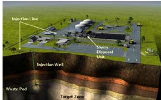
**Figure 1: Schematic of SFI Facility**
