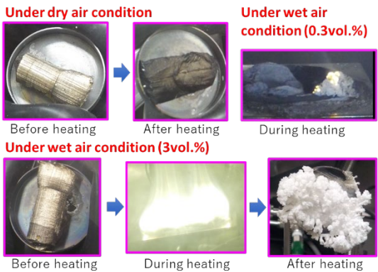
Fig. 1 The images of the heating experiments under different conditions without insulators.
