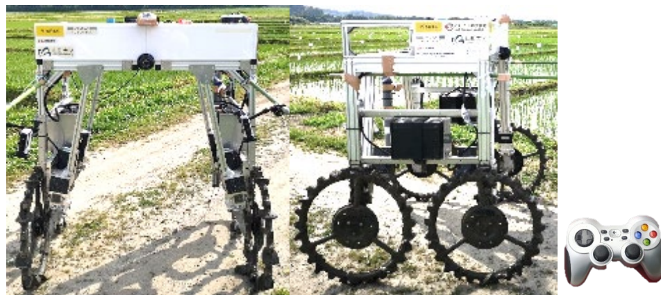
Figure 1. Front & Side view of crop sensing robot and remote controller
