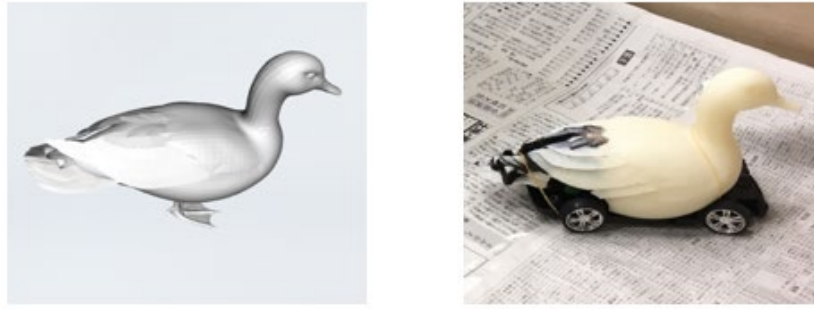
Figure 6: 3D mallard model (left) and mounting on UGV (right).
