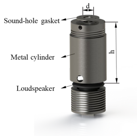
Figure 7. The schematic diagram of the loudspeaker-based excitation device. (d: the diameter of gasket; h: the distance between fruit surface and loudspeaker)
