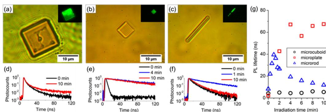
Figure 1. Optical microscope images and PL decay curves of (a, d) a microcuboid, (b, e) a microplate, and (c, f) a microrod. The insets show the PL images of the crystals. (g) The time evolutions of the PL lifetimes of the microcuboid (○), the microplate (□) and the microrod (△).
