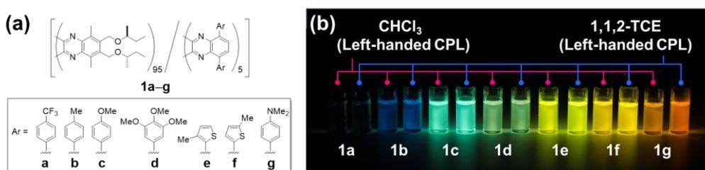
**Figure 1.** (a) Structures of **1a–g**. (b) Picture of **1a–g** in CHCl<sub>3</sub> or 1,1,2-TCE under UV-light (365 nm) irradiation.
