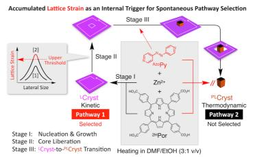
crystal, initially formed by excluding the pillar component, carries a single dislocation at its geometrical center. This crystal "spontaneous-ly" liberates a core region to relieve the accumulated lattice strain around the dislocation. Consequently, the liberated part becomes dy-namic and enables the pillar ligand to invade the crystalline lattice, thereby transforming into a thermodynamically preferred pillared-layer crystal.
