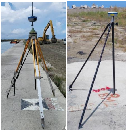
Figure 3 CHCNAV iBase as base station (left) and STONEX S9 as rover (right)
