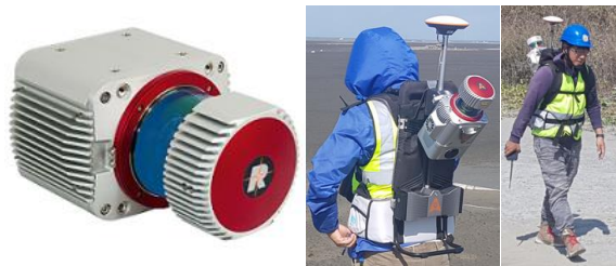
Figure 4 RIEGL VUX1UAV (left) and the use of the LiDAR strapped to Backpack on the field (right)
