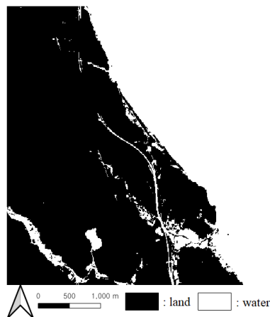
Figure 7 Binary image generated from the NDWI image
