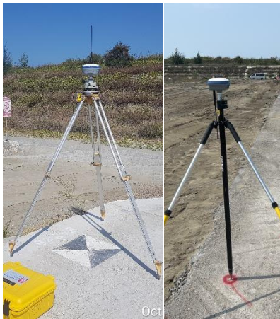
Figure 2 CHCNAV iBase as base station (left) and PrinCe i30 as rover (right)
