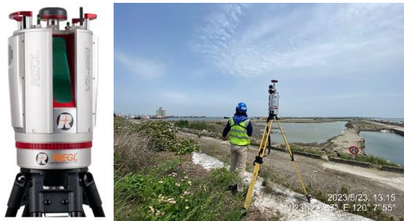
Figure 5 RIEGL VZ-400i (left) and operation of the equipment scanning the while port visible (right)
