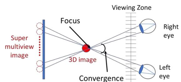
Fig. 2 Principle of Super-multiview display.
