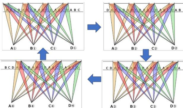
Fig. 4 Time-division quadruplexing parallax barrier.
