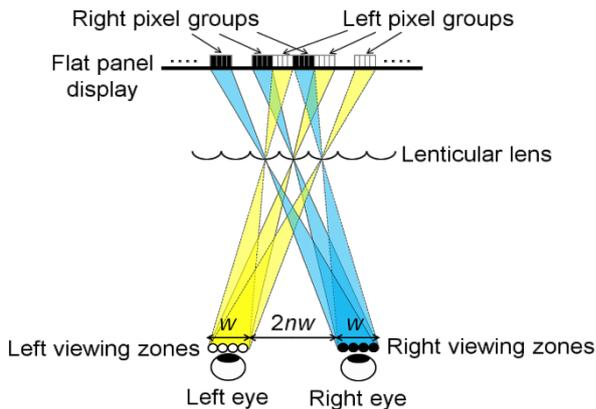
Fig. 3 Super-multiview display with head-tracking [5].
