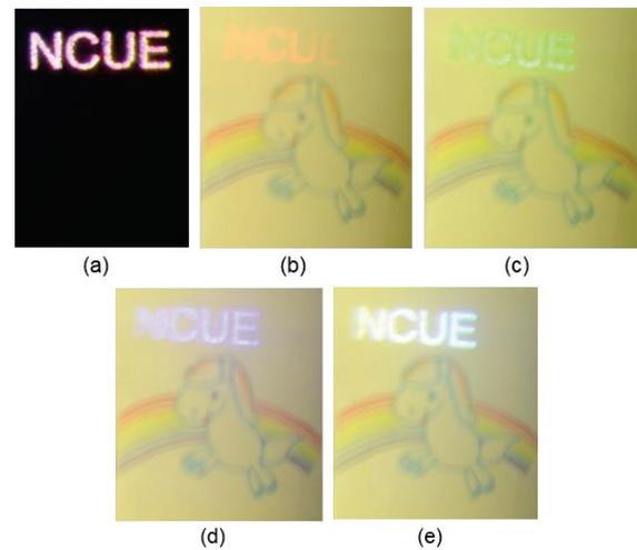
**Fig. 5. The figure shows (a) the input image after digital correction, the (b) red; (c) green; (d) blue output image and the (e) full color output image in bright room.**
