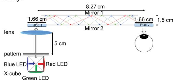
Fig. 1. The proposed system of the full color HMD based on transmission-type HOEs.
