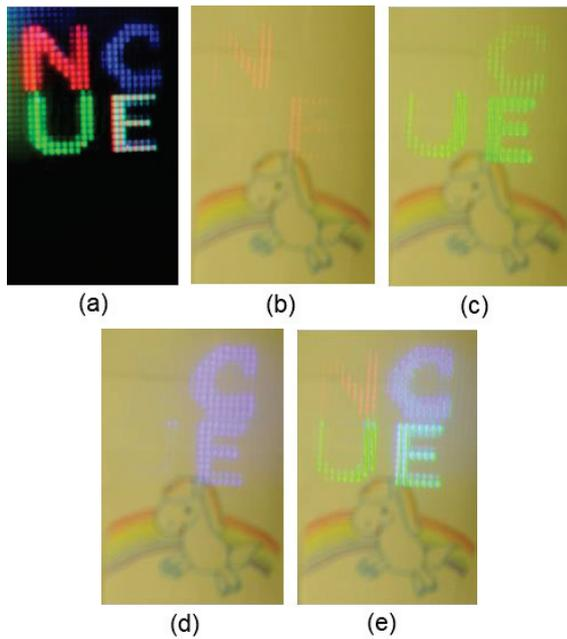
**Fig. 4. The figure shows (a) the input image by panel and white LED light source which combined by RGB LED, the (b) red; (c) green; (d) blue output image and the (e) full color output image in bright room.**
