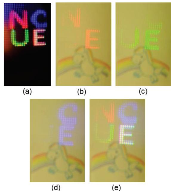
**Fig. 6. The figure shows (a) the input image after digital correction, the (b) red; (c) green; (d) blue output image and the (e) full color output image in bright room.**
