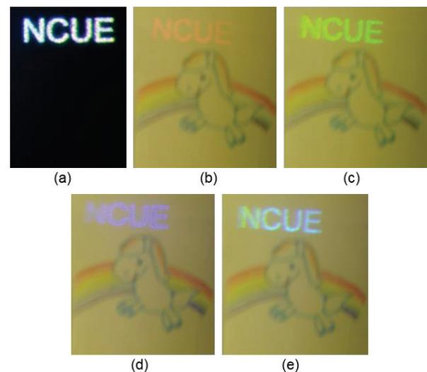
**Fig. 3. The figure shows (a) the input image by white LED light source which combined by RGB LED, the (b) red; (c) green; (d) blue output image and the (e) full color output image in bright room.**
