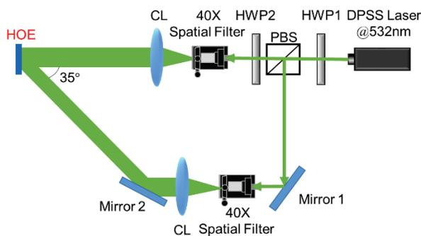
**Fig. 2. The system of recording input and output HOE.**
