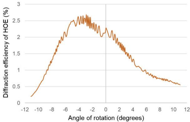
**Fig. 7. The angular sensitivity of the system.**
