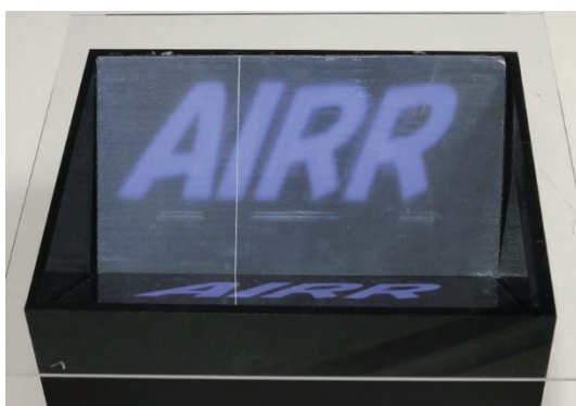
Fig. 1 Aerial image formed with AIRR (aerial imaging by retro-reflection).
