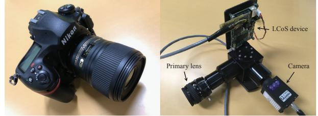
Fig. 1: Cameras used for FS (left) and CA (right) methods.
