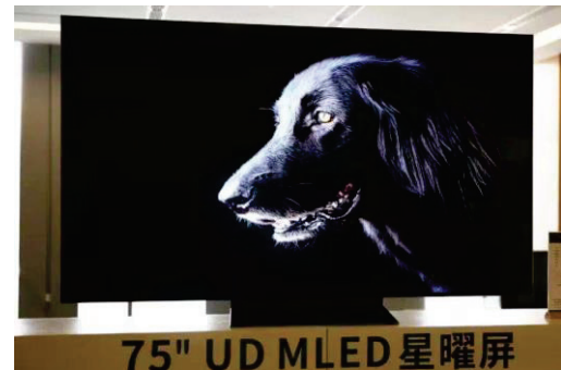
Fig.11 Demo of the 75 inch display with the AM miniLED backlight system on glass and a 4K LCD panel
