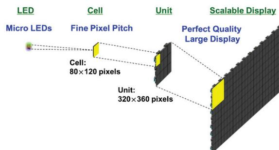
Figure 3. Structure of Crystal LED display system
