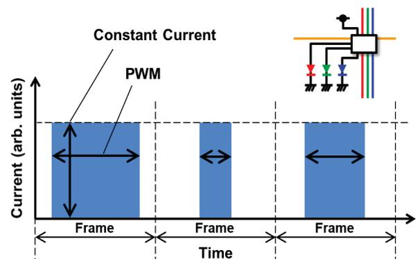
**Figure 7.** Waveform of constant current PWM of micro LED by micro IC
