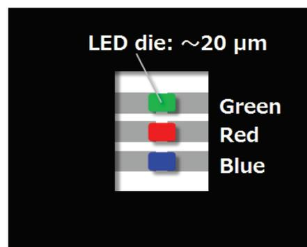
Figure 4. Micro LEDs and their pixel layout
