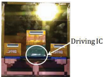
Fig. 8 Driving IC and PCBA for AM driving
