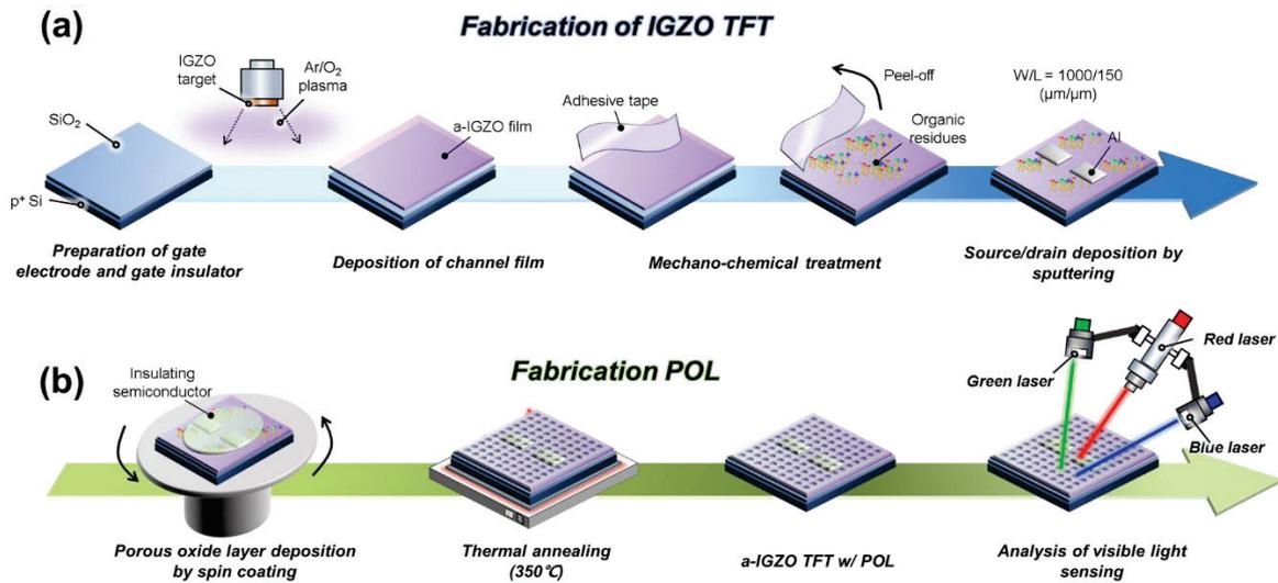
Fig. 1 Schematic diagram of fabrication process for IGZO TFT w/ POL using mechano-chemical treatment.
