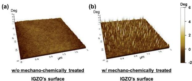
Fig. 2 The AFM analysis of IGZO films; (a) w/o treated surface of IGZO, (b) w/ treated surface of IGZO.
