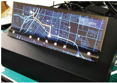
Fig. 7 Fabricated prototype flexible OLED display
