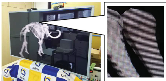
Fig. 3 Sample of 8K-UHD 3D surgical image (CG) with line by line format.
