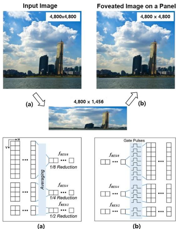
Fig. 4 The proposed driving scheme. (a) Vertical resolution reduction (b) Foveated-rendering image construction of original resolution on a panel by multi-output driving.
