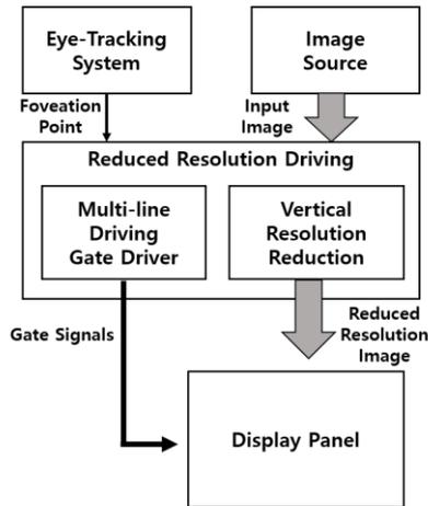
Fig. 3 Block diagram of the foveation-based reduced resolution driving scheme.
