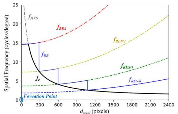
**Fig. 2** Spatial frequencies for the distance from a foveation point at the resolution of 4,800x4,800.  $\beta$  is 0.35.  $e_2$ ,  $CT_0$  and  $\alpha$  are 2.3, 1/64 and 0.106. The overlapped regions of half Nyquist frequencies are  $f_{RR}$ .
