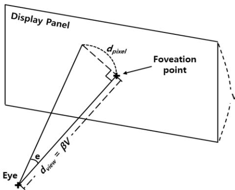
**Fig. 1** Viewing geometry for parameters of viewing distance ( $d_{view}$ ) which is the value of vertical resolution ( $V$ ), eccentricity ( $e$ ), and the distance from a foveation point ( $d_{pixel}$ ).
