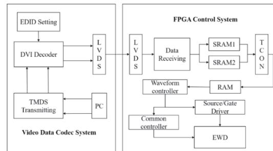
Fig. 1 The structure of EWD driving system
