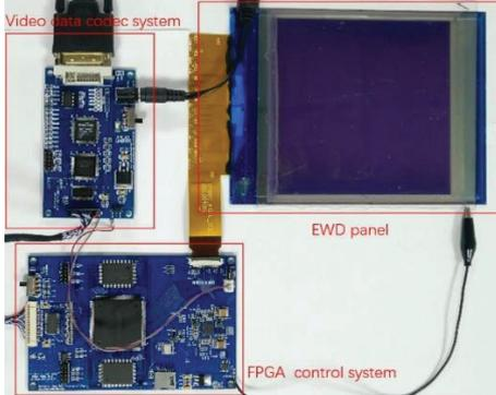
**Fig. 8 The implemented EWD driving system**
