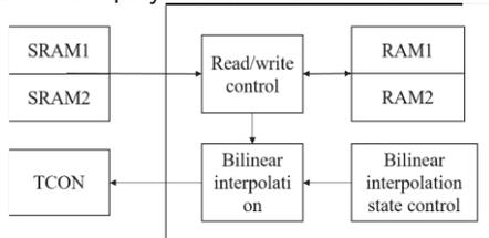
**Fig.4 The kernel structure of the bilinear interpolation**
