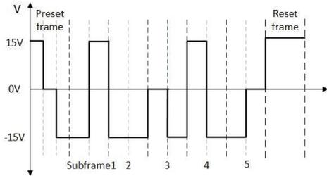
**Fig.7 Dynamic symmetric driving waveform**
