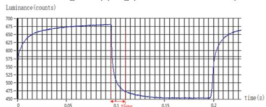
**(a)The response time under conditional driving waveform**
