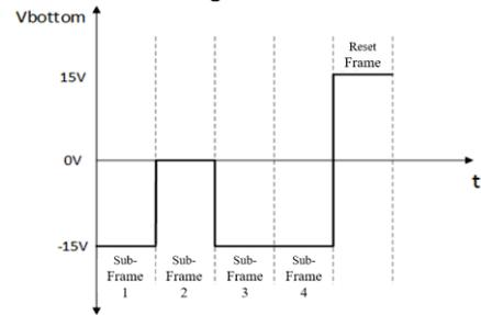
**Fig.6 Dynamic asymmetrical driving waveform of gray level 9**
