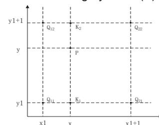
Fig. 2 Bilinear interpolation algorithm window
