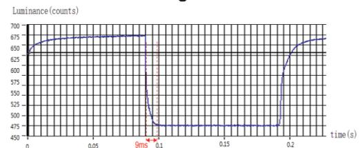
**(b)The response time under proposed driving waveform**
