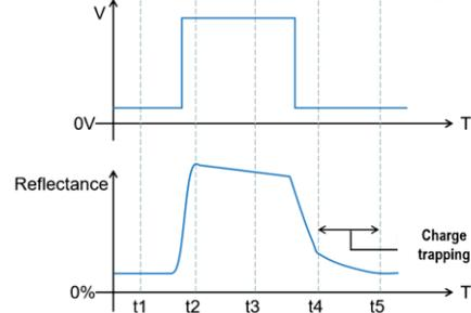
**Fig.5 Charge-trapping phenomenon of the EWD**
