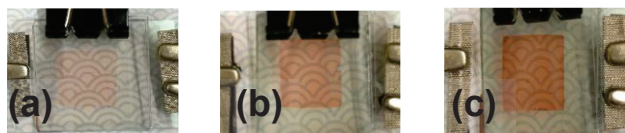
Fig. 5 Photographs of the ECDs with the ITO particle-modified counter electrodes (thickness: (a) 1.3 \mu\text{m} , (b) 4.7 \mu\text{m} and (c) 8.8 \mu\text{m} ).
