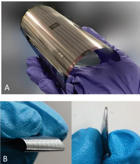
**Fig. 2** Optical images of poly-Si CMOS devices on steel after thinning to 5  $\mu\text{m}$  substrate thickness. 6x6" Sheet with the devices after thinning (A). Demonstrating bendability (B).
