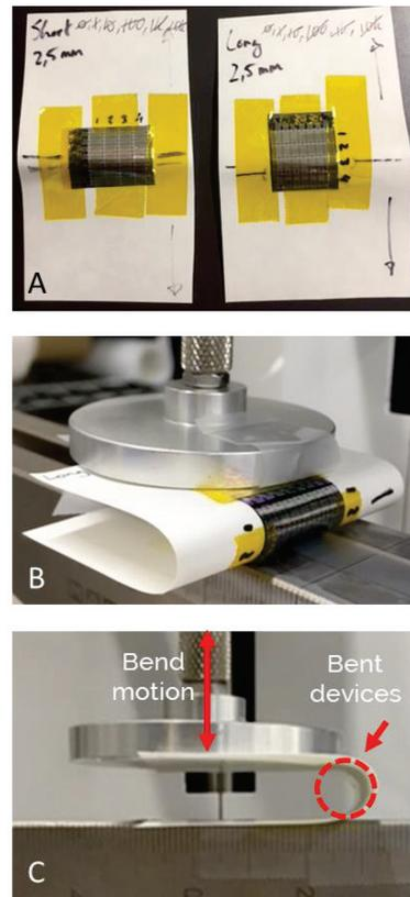
**Fig. 3** Optical images of thinned samples taped on coupons for bend tests (A), bend test configuration from an angle (B), bend test configuration from the side showing bend radius (C).
