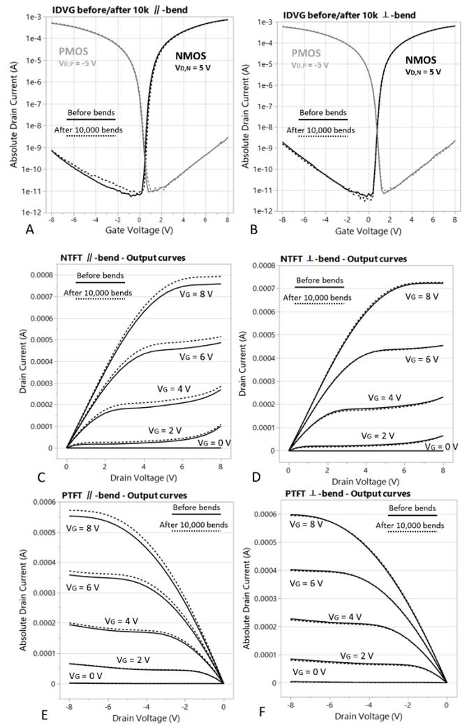
**Fig. 5 NMOS and PMOS TFT transfer and output characteristics before bends and after 10,000 bends. TFT transfer // -bend (A), and ⊥ -bend (B). TFT output. NMOS // (C) and ⊥ (D)-bend, PMOS // (E) and ⊥ (F)-bend.**
