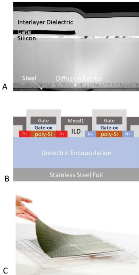
**Fig. 1** SEM image showing the barrier layer on steel (A). Schematic of CMOS TFTs fabricated on steel (B), optical image of NFC devices fabricated on a flexible stainless steel sheet (C).
