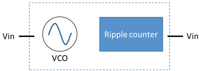
Fig. 1 Schematic of VCO based ADC
