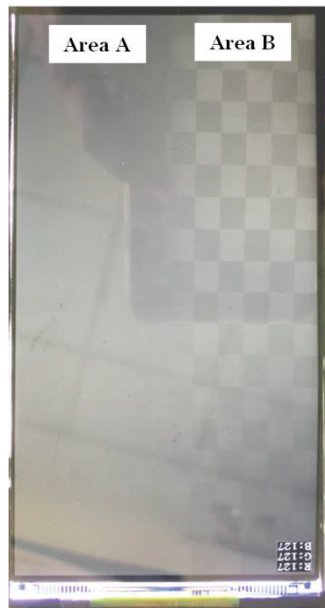
Photo. 2 Image sticking phenomenon of two areas IS level before and after irradiation
