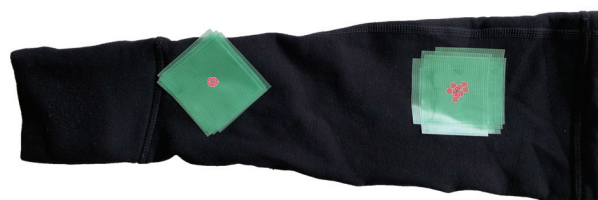
Figure 5. The positions of the two electrode modules for right forearm.
