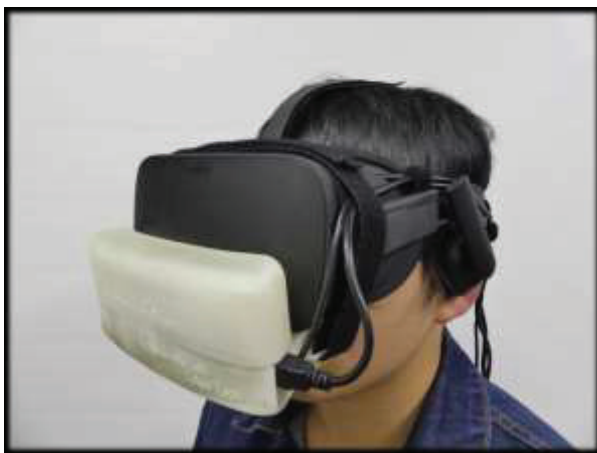
Fig.5 Photo of wearable olfactory display (white one) attached to HMD.
