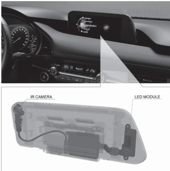
**Fig.7 Driver monitor camera in CID**
