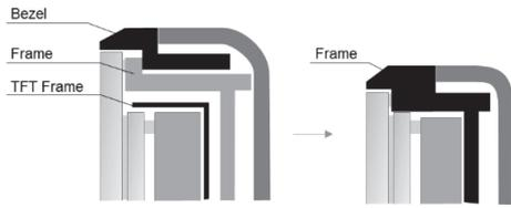
**Fig.6 Narrow border structure**
