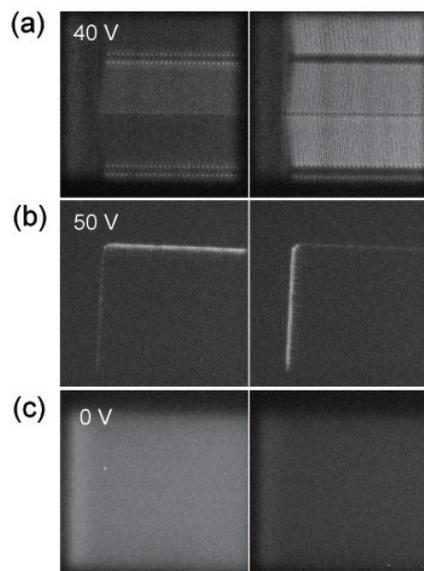
Fig. 3 SH micrographs of 5CB for various liquid crystal cells. (A) n-type mixture in an FFS cell with a voltage of 40 V, (b) 5CB in a TN cell with a voltage of 50 V, and (c) 5CB in a wedge cell without an electric field. The incident polarization is vertical (left column) and horizontal (right column).
