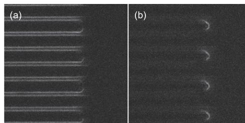
Fig. 2 SH micrographs taken for 5CB in an in-plane electrode cell by applying a square wave with amplitude of 50 V. The incident polarization is (a) vertical and (b) horizontal.
