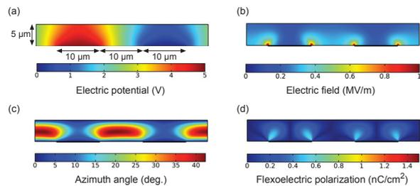
Fig. 4 Simulation results of an IPS cell with n-type nematic liquid crystals. (a) Electric potential, (b) Electric field, (c) Azimuth angle of the director and (d) Flexoelectric polarization.
