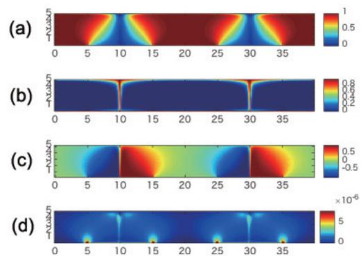
Fig. 5 Simulation results of an IPS cell with p-type nematic liquid crystals at an applied voltage of 50V. (a) x component ( $n_x$ ), (b) y component ( $n_y$ ), (c) z component ( $n_z$ ) of director and (d) Flexoelectric polarization ( $|P|$  [ $C/m^2$ ]).
