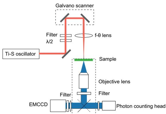
Fig. 1 Optical setup for SHG microscopy.
