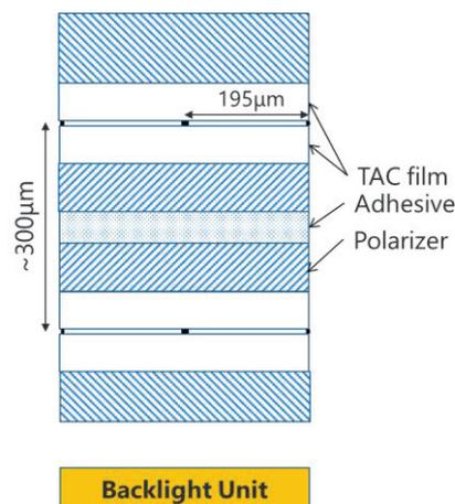
Fig. 3 OLCD dual cell test structure comprising two monochrome dual cells of the same design
