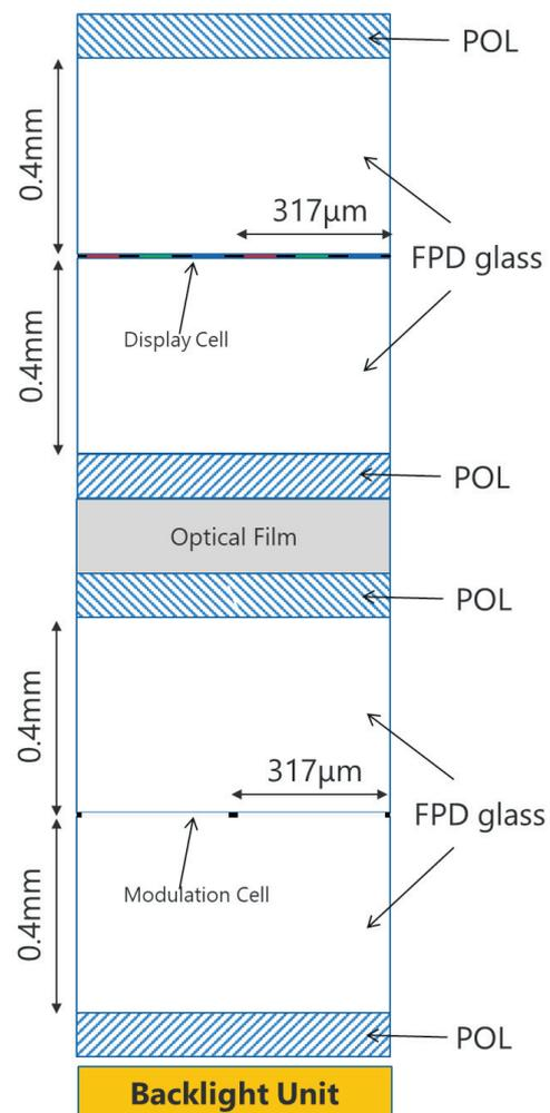
**Fig. 1 Schematic glass Dual Cell structure drawn to scale for a 4K 55" TV, to illustrate the large inter-cell separation relative to pixel pitch**
