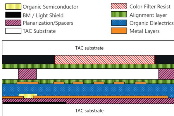
Fig. 2 Schematic OLCD stack using TAC substrate
