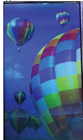
Fig. 6 4.99" 294ppi AOC with PDLC panel light on image.
