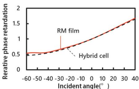
**Fig. 4 Incident angle-retardation characteristics of RM film.**
