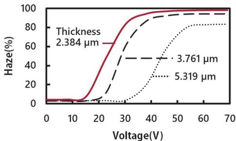
**Fig. 3 Voltage-haze characteristics when the coating thickness of UV-polymerized monomer changes.**
