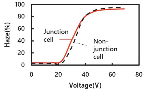
**Fig.7 Comparison of haze characteristics of junction cell and non-junction cell.**
