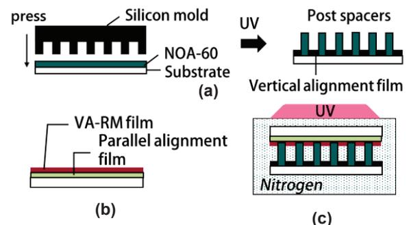
Fig. 2 Fabrication process. (a) Post spacer transfer. (b) Apply RM on parallel alignment film. (c) UV irradiation under nitrogen atmosphere after superposition.
