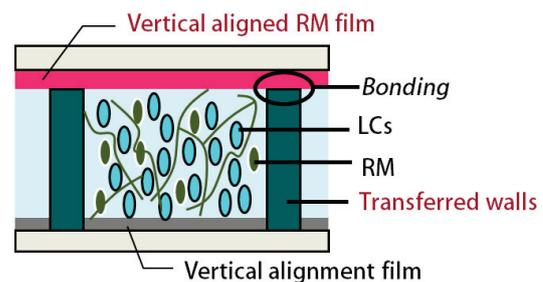
Fig. 1 Schematic diagram of PNLC cell structure with bonding transferred spacers.
