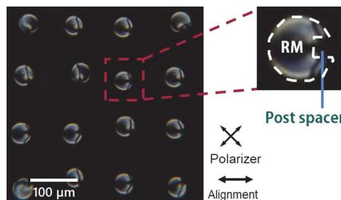
**Fig. 5 Appearance of junction cell after UV curing without liquid crystal.**
