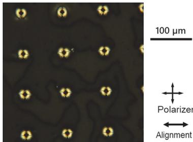
**Fig. 6 Appearance of a junction cell fabricated using RN-3222 after liquid crystal injection.**
