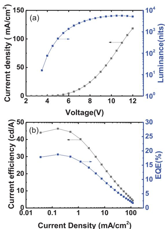
Figure 2. (a) current density and luminance versus voltage, (b) current efficient and external quantum efficiency versus current density of OLED with FIrpic emitter.
