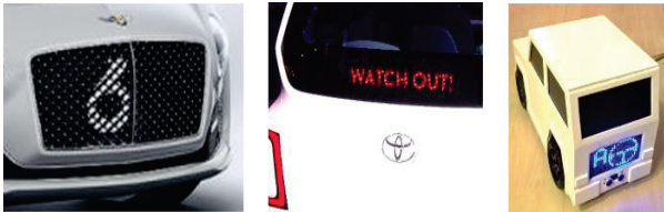
Fig. 10 Prototypes of exterior displays for autonomous cars: Front display with low resolution (left) and rear displays for characters (center) and icons (right, model car [5]).
