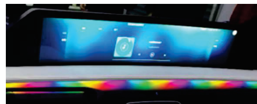
Fig. 8 Full color light effects (grey level, width, direction, speed, ramp ...) by direct-lit "pixelated" light guide.
