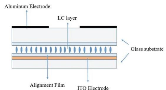
**Fig. 1 Structure of UV<sup>2</sup>A nematic LC lens.**
