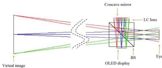
Fig.5 Optical system for augmented reality
