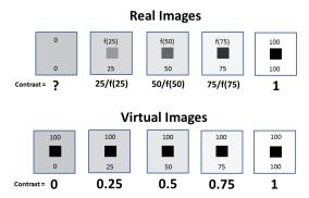
Fig. 1 comparison of contrast ratio methods for PM2.5 measurements using projection images [4]
