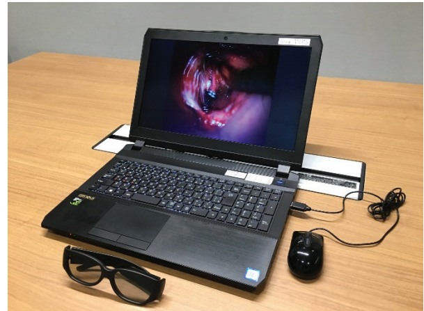
Fig. 7 Down-converted 4K3D image displayed on the developed 15.6" 4K3D notebook PC.
