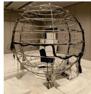
Fig. 6 Equipment for measuring emission characteristics from sound source
