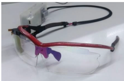
Fig. 6 Prototype of full-color AR glass with HOE waveguide on a plastic substrate
