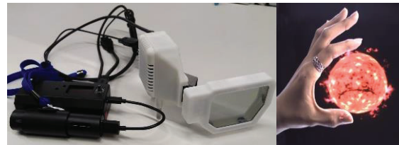
Fig. 7 Prototype of full-color laser beam scanning based retinal scan near-eye display and image displayed through the prototype
