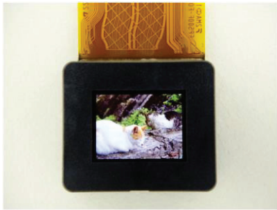
Fig. 5 0.5" 4032-ppi OLED microdisplay with 6.3- \mu\text{m} pixel size and 1.6 K \times 1.2 K pixels
