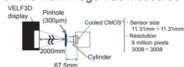
Fig. 4 Measurement of luminance distribution of VELF3D display
