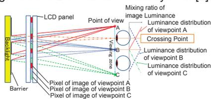
Fig. 2 Mechanism of VELF3D display
