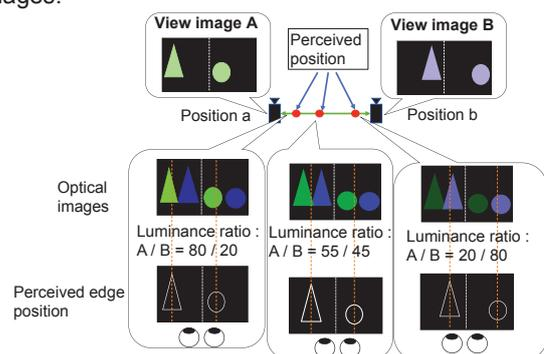
Fig. 1 Schematic illustration of linear blending technology
