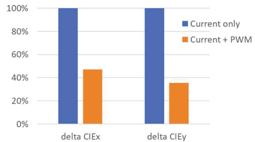
Fig. 4. Relative CIE chromaticity variation of green microLED emission for current-only driving vs. current and PWM hybrid driving.
