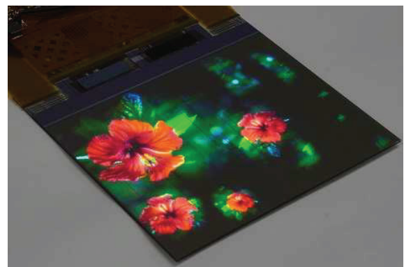
Fig. 9. Photograph of 3.9" microLED display prototype.
