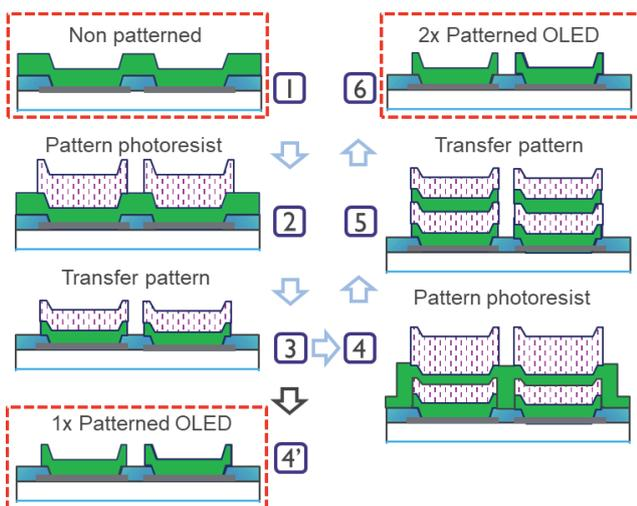
**Fig 2. The schematic flow to fabricate non-patterned, 1x patterned, 2x patterned samples**
