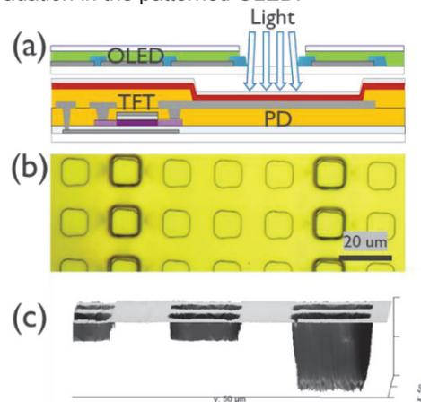
**Fig 6. (a) The schematic of the under-display imager application with OLED stack with hole openings (b) Microscope image of an OLED array with hole openings (c) AFM image of the patterned OLED stacks**
