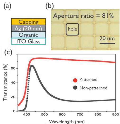
**Fig 5. (a) Schematic of organic/Ag/Capping stack to be patterned (b) microscope image of patterned stack (c) transmission spectra of patterned and non-patterned samples**
