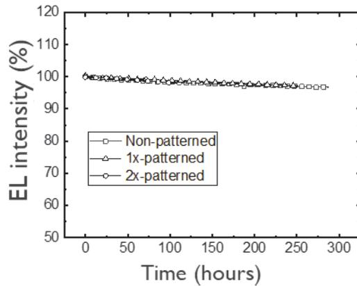
**Fig 4. OLED device lifetime at 1000nit of non-patterned, 1x patterned, and 2x patterned devices, respectively.**
