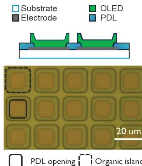
**Fig 1. Schematic and microscope image of OLED islands on top of the PDL opening.**
