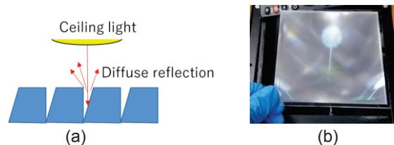
**Fig. 4. Diffuse reflection caused at the groove of the DCRA.**
