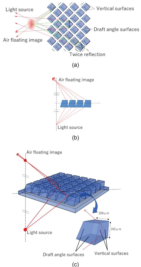
**Fig. 1. Schematic illustration of the transparent material type DCRA and rays.**
