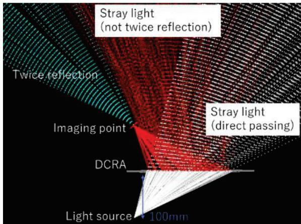
**Fig. 3 Side view of DCRA and its ray tracing simulation.**
