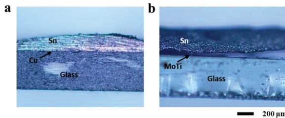
**Fig. 4** Optical microscope images (a) Cu and (b) MoTi film after reflow soldering on cross-section views.
