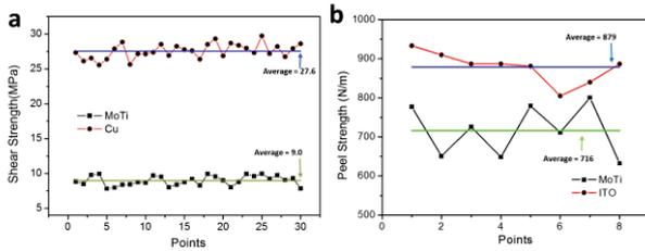
**Fig. 3** (a) Shear bond strength of LED, (b) peel strength of COF bonding area.
