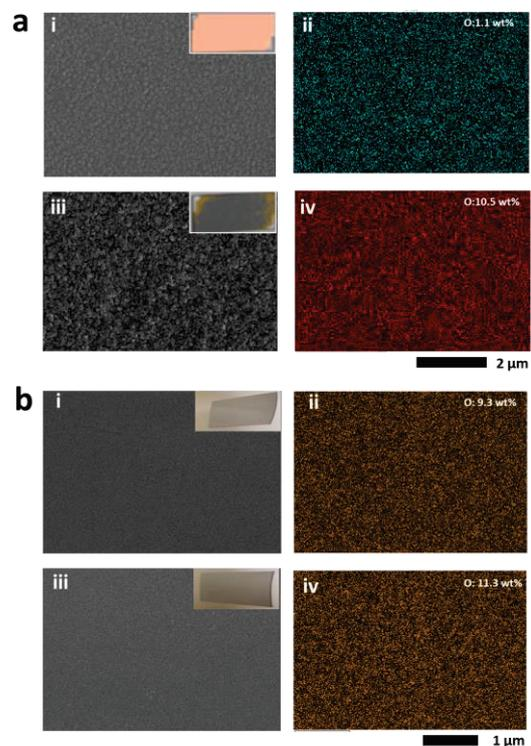
**Fig.2** Scanning electron microscope images and EDS mapping of the surface O elements before (i, ii) and after (iii, iv) heating at 250 °C for 2 h: (a) Cu, (b) MoTi.
