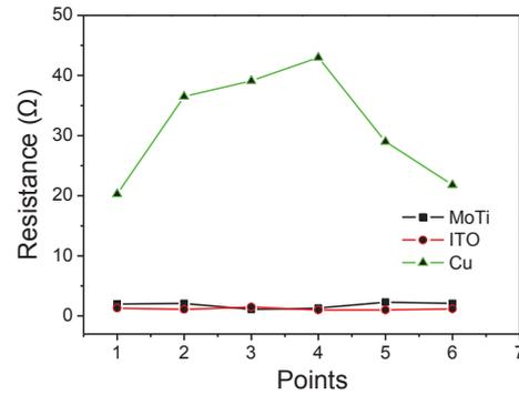
**Fig.5** Resistance between COF and different metal film.
