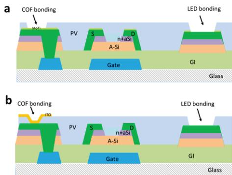
**Fig.1** Schematic cross section of a mini-LED backlight TFT: (a) 4-Mask TFT, (b) 5-Mask TFT.
