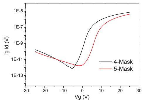
**Fig.6** Transfer characteristics of miniled backlight TFTs with MoTi/Cu/MoTi and Cu as Source/Drain.
