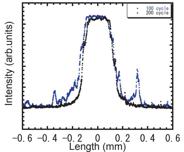
Fig. 5. Transverse line profiles of surface pictures for micro-LEDs embedded in shallow and deep Si micro-cup substrates.
