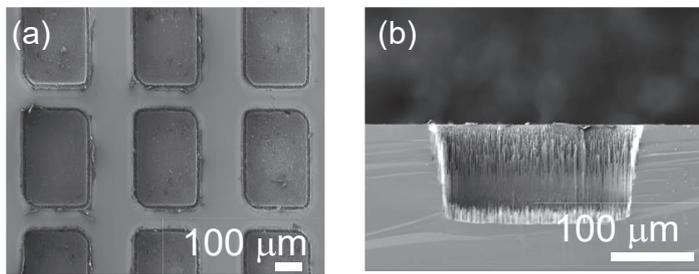
Fig. 2. (a) Surface and (b) transverse cross-sectional SEM images of Si micro-cup formed by 200 cycles of BOSCH process.
