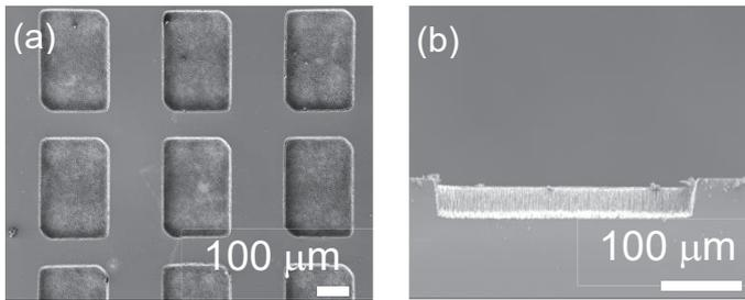
Fig. 1. (a) Surface and (b) longitudinal cross-sectional SEM images of Si micro-cup formed by 100 cycles of BOSCH process.
