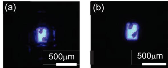
Fig. 4. Emission patterns of micro-LEDs embedded in (a) shallow and (b) deep Si micro-cup substrates.
