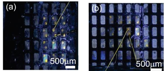
Fig. 3. Surface pictures of micro-LEDs embedded in (a) shallow and (b) deep Si micro-cup substrates.
