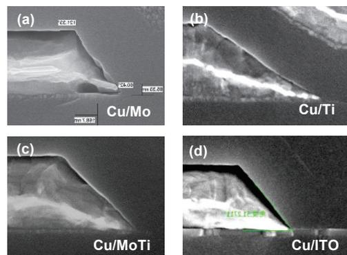
**Fig. 4** Undercut and Cu loss phenomenon with the barrier material (a) Mo, (b) Ti, (c) MoTi alloy and (d) ITO.
