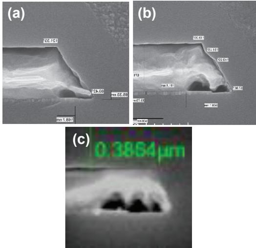
**Fig. 2** Different degree of Mo undercut and Cu loss after T300 station with (a) one Cu empty hole, (b) two Cu empty holes and (c) three Cu empty holes.
