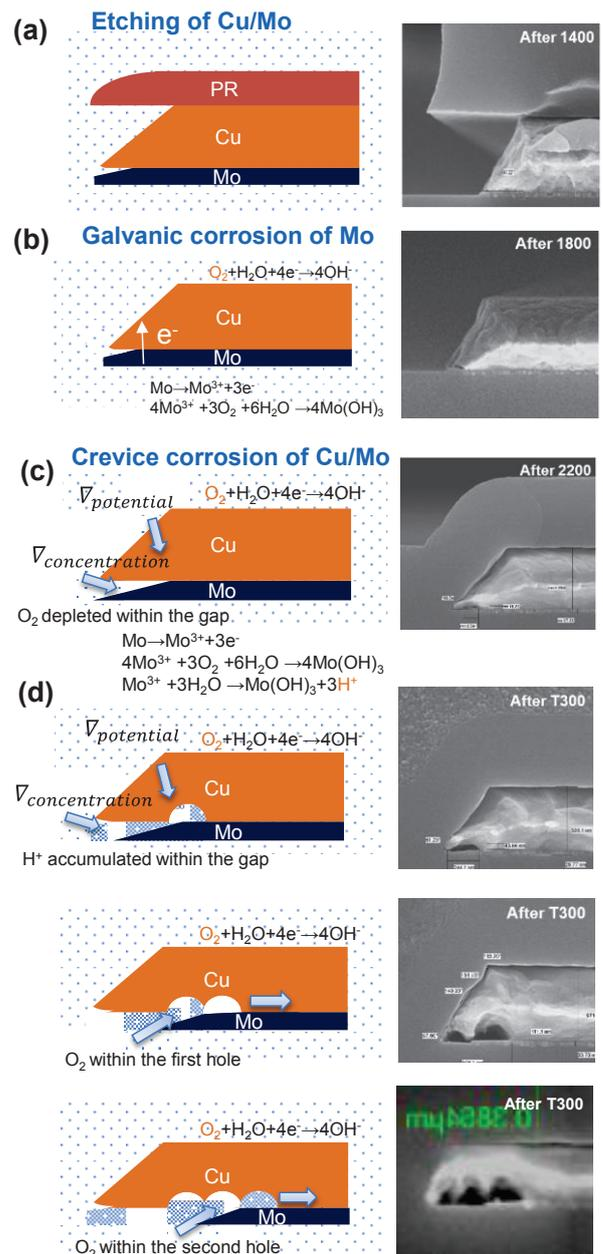
**Fig. 3** The proposed mechanism of the formation of Mo undercut and Cu loss.
