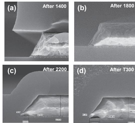
**Fig. 1** The formation of Mo undercut and Cu loss during manufacturing process of LCD display with the respectively taper morphology after (a) wet etching (1400 station), (b) stripper of photoresist (1800 station), (c) gate insulator deposition (2200 station) and (d) array test (T300 station).
